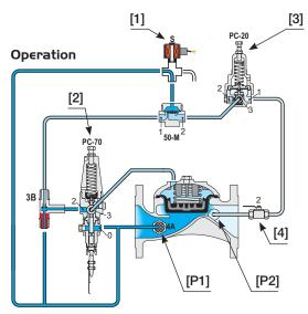
Energizing the Solenoid [1] opens the valve. The Flow Pilot [2] commands the valve to throttle closed should demand rise above setting, and to modulate open when demand drops. The Pressure Reducing Pilot [3] controls the valve, preventing Downstream Pressure [P2] from rising above setting. De-energizing the solenoid causes the valve to shut. The downstream Cock Valve [4] enables manual closing.
